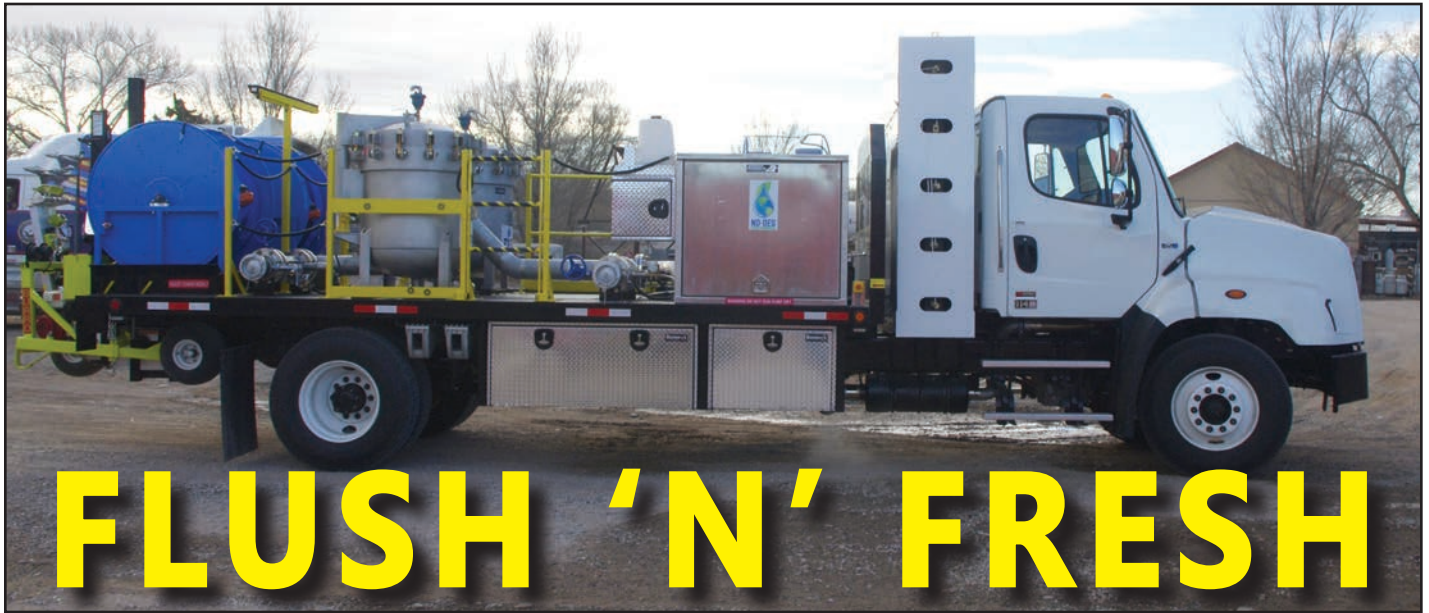
The Neutral Output Discharge Elimination System, NO-DES, truck is fully equipped with the controls, pumps, filters, hoses and necessary components to flush and filter a potable water system. Photo courtesy of NO-DES Inc.
